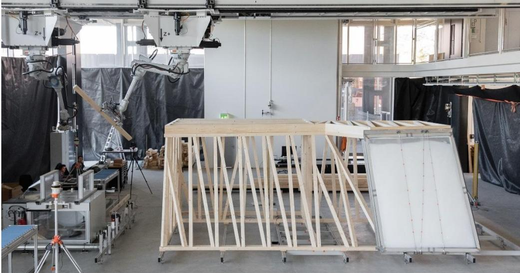
*Robotic Assembly of a Timber Frame Module, ETH Zurich, 2017 (Photo Credit: Gramazio Kohler Research)*
